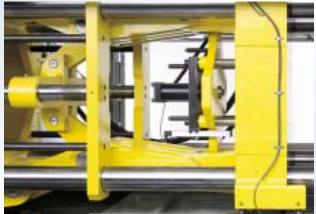
Recent clamp improvements include a strengthened crosshead and ejector plate for durability and guidance.
