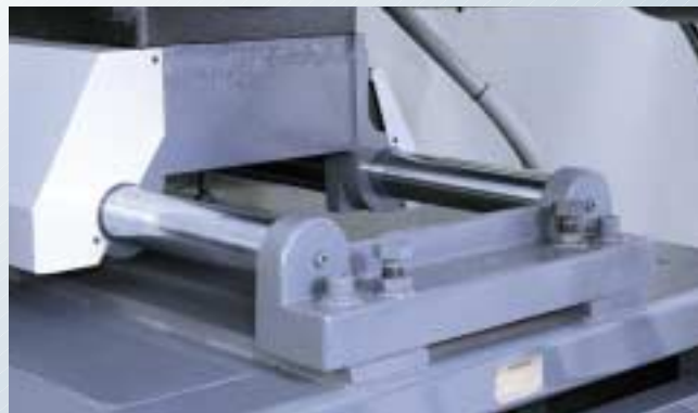
The injection carriage is supported on round guide rods providing 360-degree containment of the bars. It accommodates both standard and long L/D screws and barrels.
