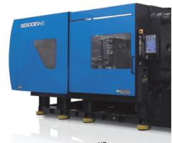
[Above] The 562 U.S. ton SEEV-A<sup>HD</sup> machine is the largest all-electric machine the company has ever brought to an NPE.
